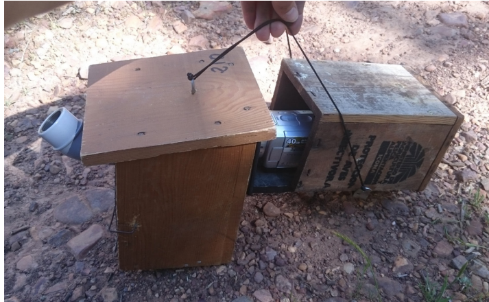
Fig. 1s. Camera-adapted nest boxes used during the study to record the diet of blue tit offspring. Regular nest-boxes were replaced with camera-adapted nest-boxes the day before the recording date.
